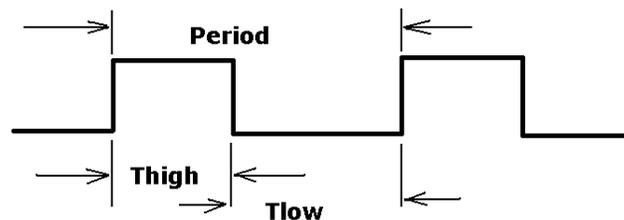
Figure 7: Oscillator period which is made of  $T_{high}$  and  $T_{low}$  pulse widths and  $1/\text{period}$  is the oscillator frequency, which is measured in all discussed sensors that produce frequency as output signal.
