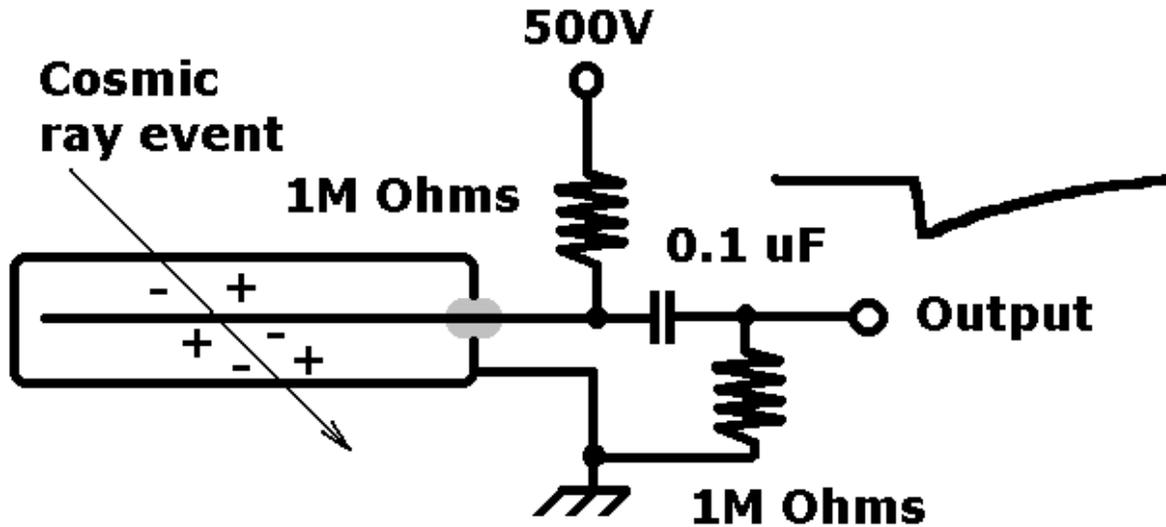
Figure 16: GM Tube cosmic ray event counting detector
